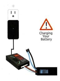
Do not leave a charging battery unattended. Unplug battery when not in use, over discharge may result in fire. When motor slows, discontinue use.
